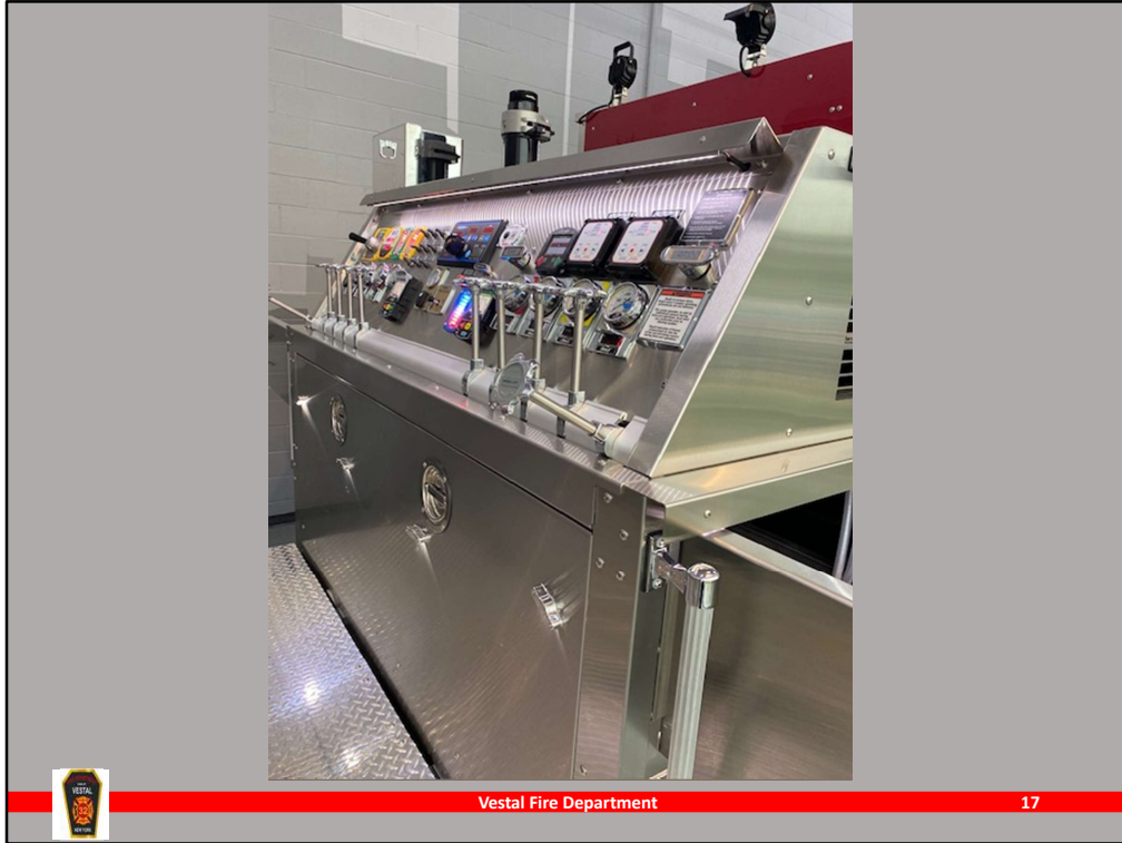
Pump Panel Area of new engine being built
